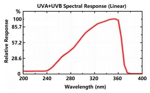
The peak point (calibration point) of UVA+B sensor spectral response is at 352 nm.
