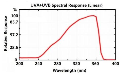
The peak point (calibration point) of UVA+B sensor spectral response is at 352 nm.
